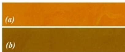
Figure 2. Radiochromic film strips: not exposed or background (a) and exposed (b).
